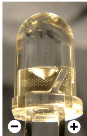
Figure 2: Polarity Determination of and LED
