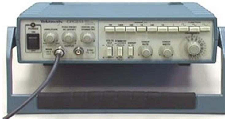
Figure 3.2: The Tektronix CFG250 Function Generator
