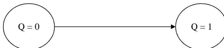
Figure 2.4: State Diagram representing a change from State Q = 0 to State Q = 1 .
