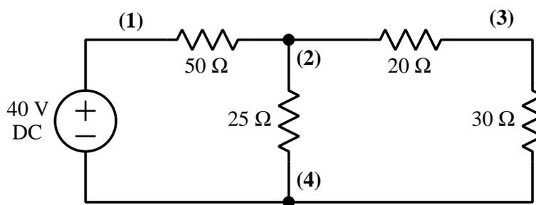
Figure 1: A Resistive Ladder Circuit
