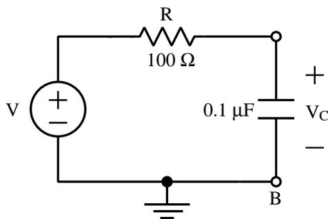
Figure 1: A Series RC Circuit
