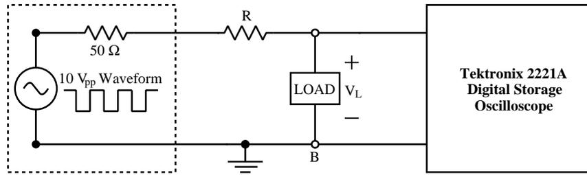
Figure 2: Generic Test Circuit
