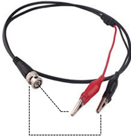
**Figure A-7:** BNC-to-alligators cable, providing two parallel electrical paths. The black alligator clip forms an electrical path with the cable's outer conductor and the BNC connector's body. The red alligator clip forms an electrical path with the cable's center conductor and the BNC connector's bayonet.
