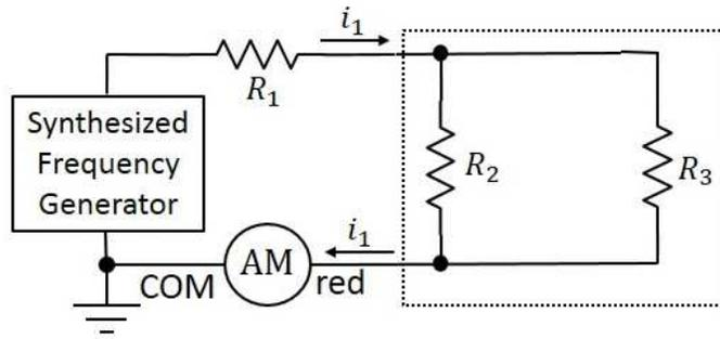
**Figure 9:** Measuring rms current  $i_1$  through  $R_1$
