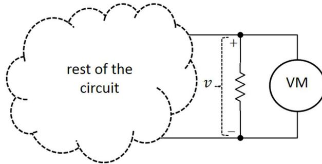
**Figure 3:** Connecting a voltmeter in parallel
