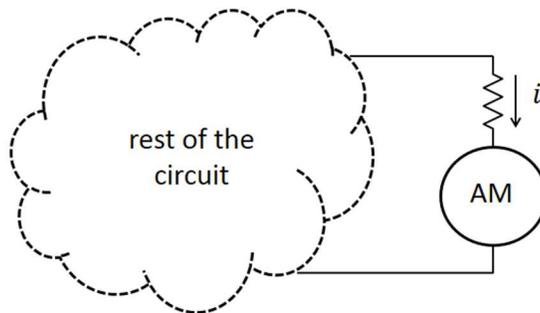
**Figure 5:** Connecting an ammeter in series
