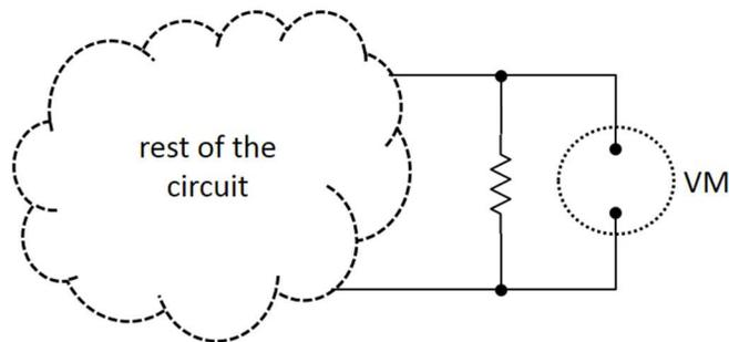
**Figure 4:** Voltmeter as viewed from the circuit
