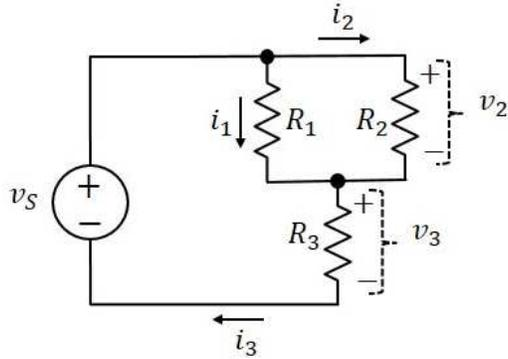
**Figure 1:** Resistive circuit with DC source
