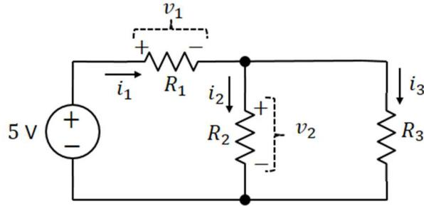
**Figure 2:** Circuit with DC source
