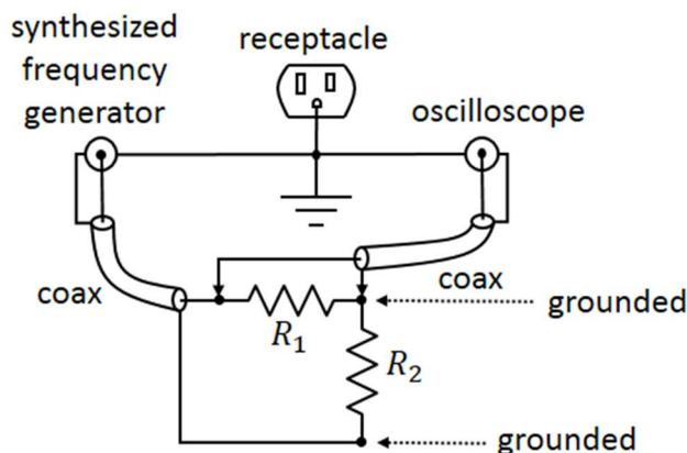
**Figure 8:** Incorrect connection of oscilloscope
