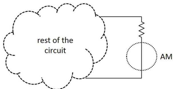
**Figure 6:** Ammeter as viewed from the circuit
