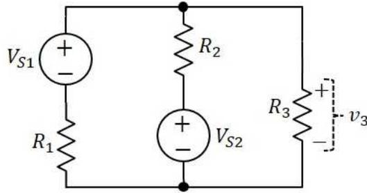
**Figure 1:** Example circuit with two DC voltage sources
