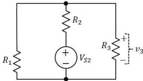
**Figure 3:**  $V_{S1}$  of Figure 1 has been set to 0
