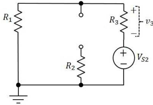
**Figure 8:** AC source of Figure 1 has been set to 0
