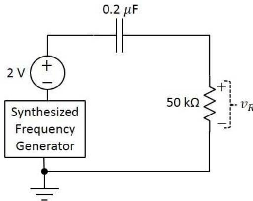
**Figure 9:** Circuit with a DC and AC voltage sources, capacitor, and resistor
