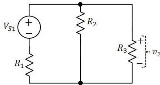
**Figure 2:**  $V_{S2}$  of Figure 1 has been set to 0
