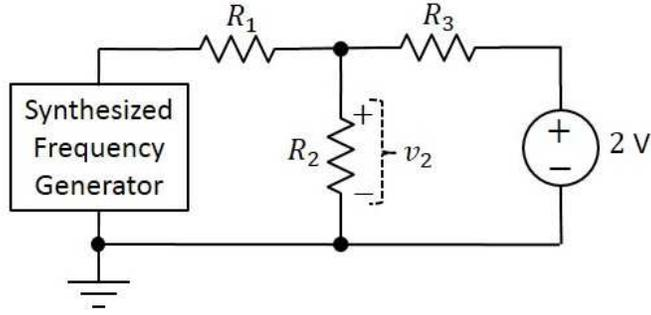
**Figure 5:** Circuit with one AC and one DC voltage source
