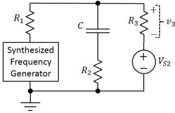
**Figure 6:** Superposition for circuit with capacitor and resistors
