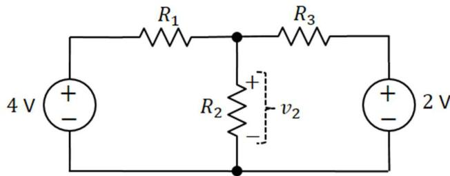
**Figure 4:** Circuit with two DC voltage sources
