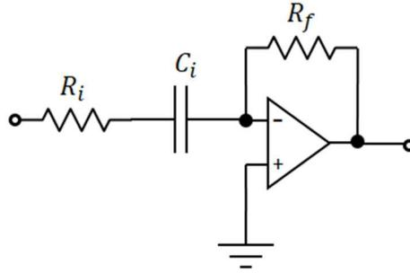
**Figure 5:** Practical differentiator (with addition of series resistor  $R_i$ )
