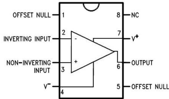
**Figure 3:** LM741 pin-out
