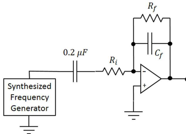
**Figure 4:** Practical integrator (with addition of feedback resistor  $R_f$ ), receiving input through a capacitor
