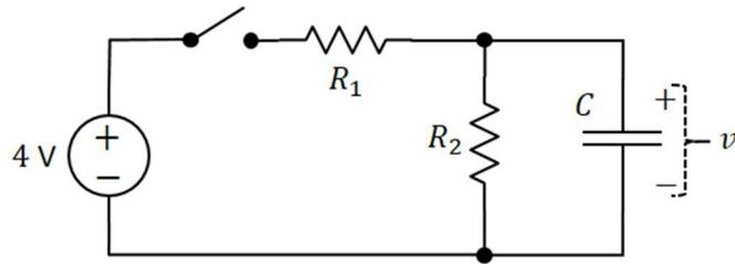
**Figure 2:** Second RC circuit
