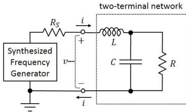
**Figure 4:** Testing the two-terminal network
