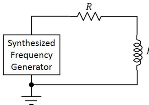
**Figure 2:** *RL* circuit
