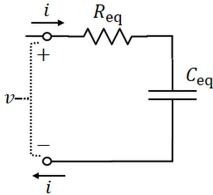
**Figure 5:** Equivalent network (for 2 kHz)
