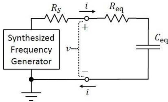
**Figure 6:** Testing the equivalent, frequency-specific network
